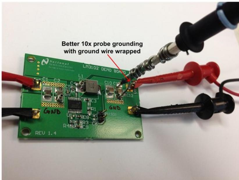
Let's compare the two probes. Here is a scope shot showing measurements taken with large ground loop probe vs the ground wire wrapped around the probe:
