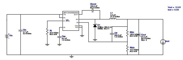
1. This regulator device is qualified for Automotive applications. All passives and other components selected in this design may not be qualified for Automotive applications. The user is required to verify that all components in the design meet the qualification and safety requirements for their specific application. View WEBENCH(R) Disclaimer.
