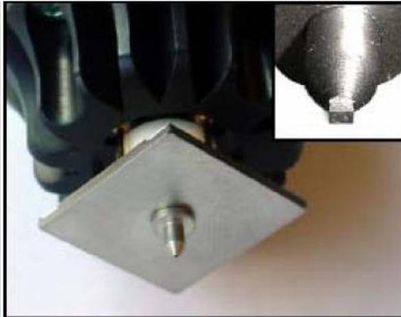
b) Electrical Conduction Nozzle
