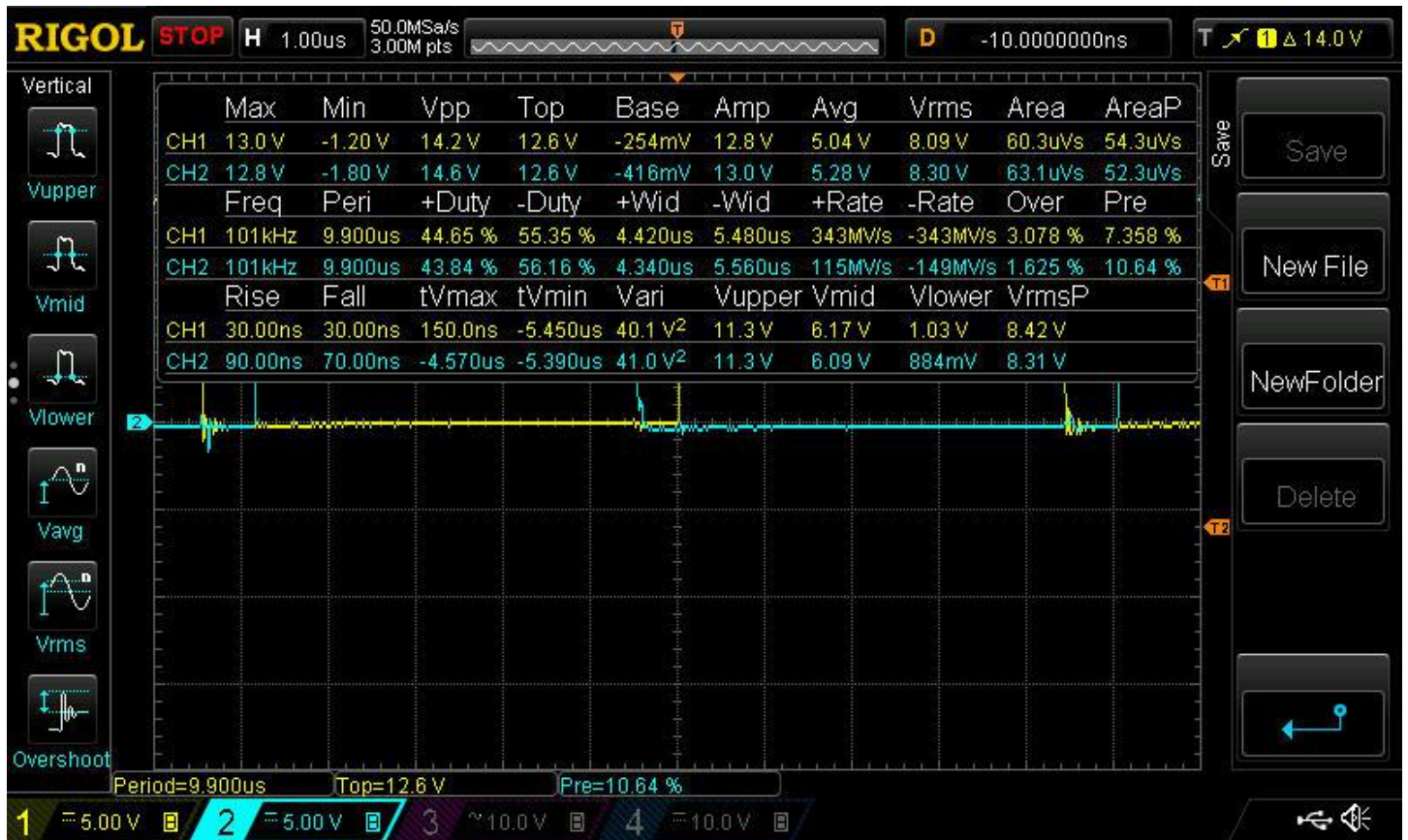
FIGURE 7 - 24mar20 2350 PIN22 OUTA - PIN21 OUTB SIGNALS
