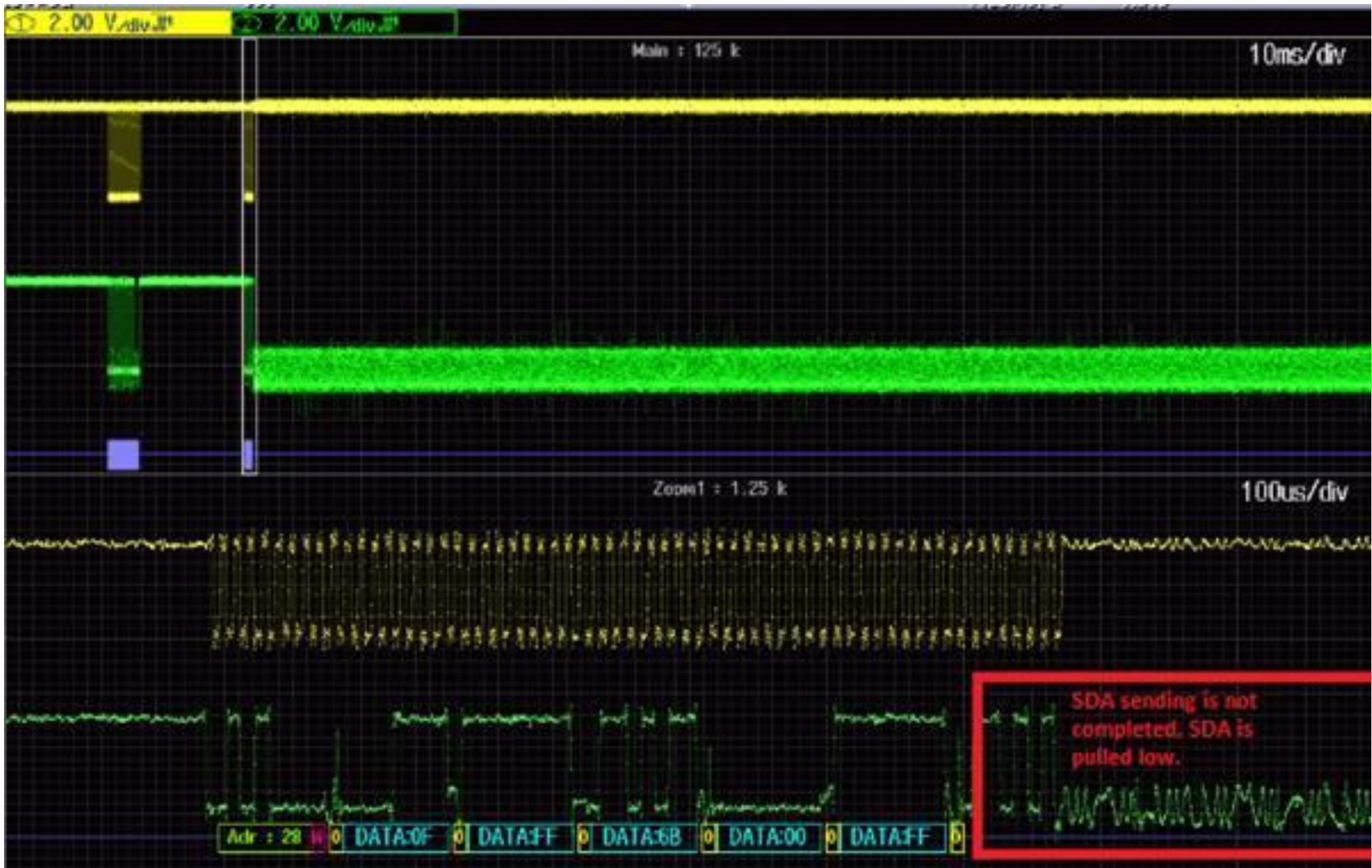
(waveform 2): SDA is not complete sending, SDA is pulled low with ripple. For this case, we need to know why the SDA is pulled low by LED driver.
