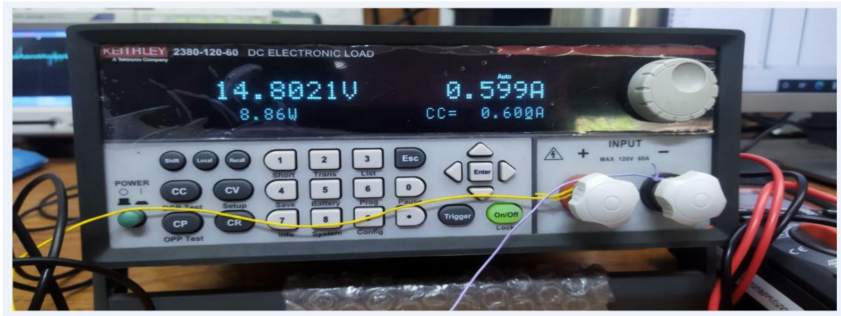
Figure 8: SMPS PCB board and Electronic load under 0.6A loaded condition.
