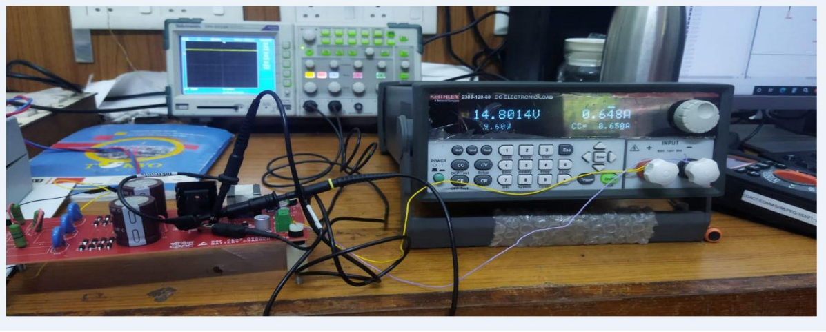
Figure 11: SMPS PCB board and Electronic load under 0.65A loaded condition.
