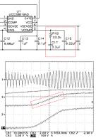
Figure 12. Start-Up Waveform (115 VAC, 60 Hz, 0.45 Å load. Ch1 = I<sub>IN</sub> @ 5 Å/dlv, Ch.2 = VCOMP @ 2 V/dlv, Ch.3 = VSENSE @ 5 V/dlv, Ch.4 = VOUT @ 100 V/dlv offset by 155 VDC)
