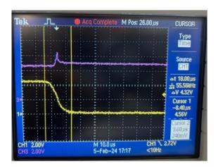
Where in this image yellow line (channel 1) = Cout pin voltage level, purple line (channel 3)= BAT pin voltage level.
