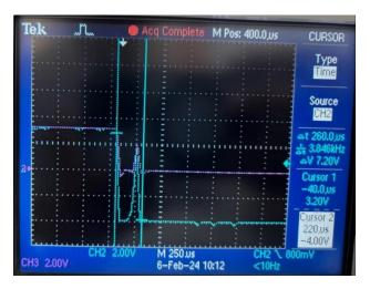
Where in this image Sky-blue line (channel 2) = Dout pin voltage level, purple line (channel 3)= BAT pin voltage level.
