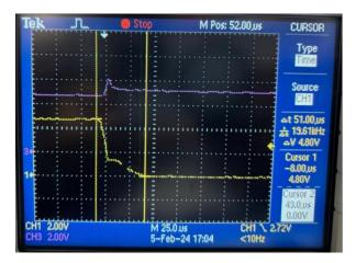
Where in this image yellow line (channel 1) = Cout pin voltage level, purple line (channel 3)= BAT pin voltage level.
