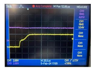
Where in this image yellow line (channel 1) = Cout pin voltage level, purple line (channel 3) = BAT pin voltage level.
