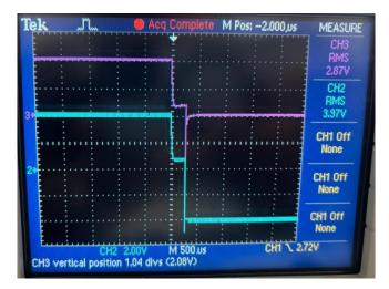
Where in this image Sky-blue line (channel 2) = Dout pin voltage level, purple line (channel 3) = BAT pin voltage level.
