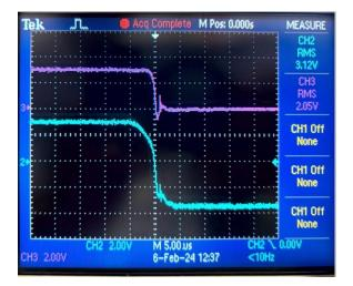
Where in this image Sky-blue line (channel 2) = Dout pin voltage level, purple line (channel 3) = BAT pin voltage level.
