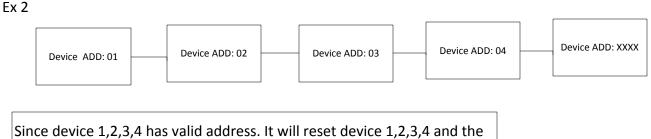
Since device 1,2,3,4 has valid address. It will reset device 1,2,3,4 and the next higher deivce (device5).
