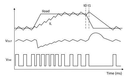
Figure 8. Load Transient Response of D-CAP3 Converter
