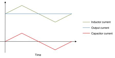
Figure 5. Current in the Buck Converter
