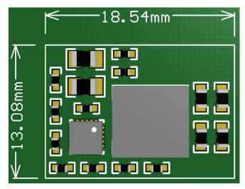
Figure 11. PCB Solution, F<sub>sw</sub> = 600 kHz
