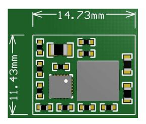
Figure 12. PCB Solution, F<sub>sw</sub> = 1000 kHz
