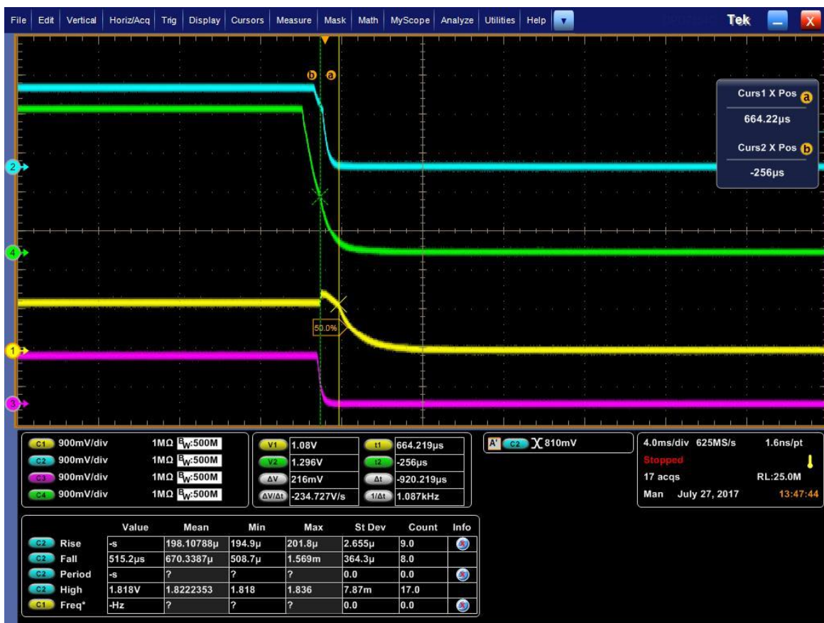
EVM, 5.0V connected to the AC input (J3/AC), power-off sequence pushing the PB_IN switch;
