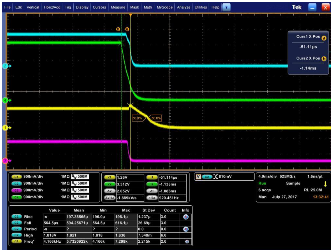
EVM, 5.0V connected to the AC input (J3/AC), power-off sequence disconnecting the 5.0V;
