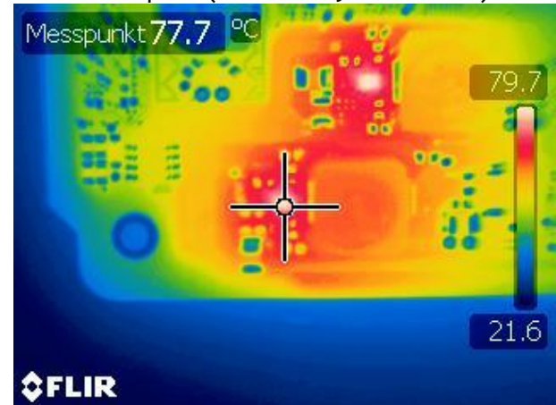
IC8 hot spot (Vout 12V, LMR36015)
