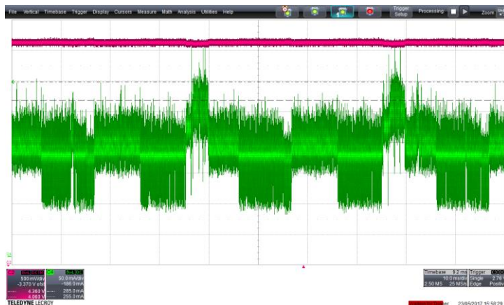
Fig.1. Red CHL: Vin; Green CHL: I+3v3_standby.50mA/div;10ms/div;
