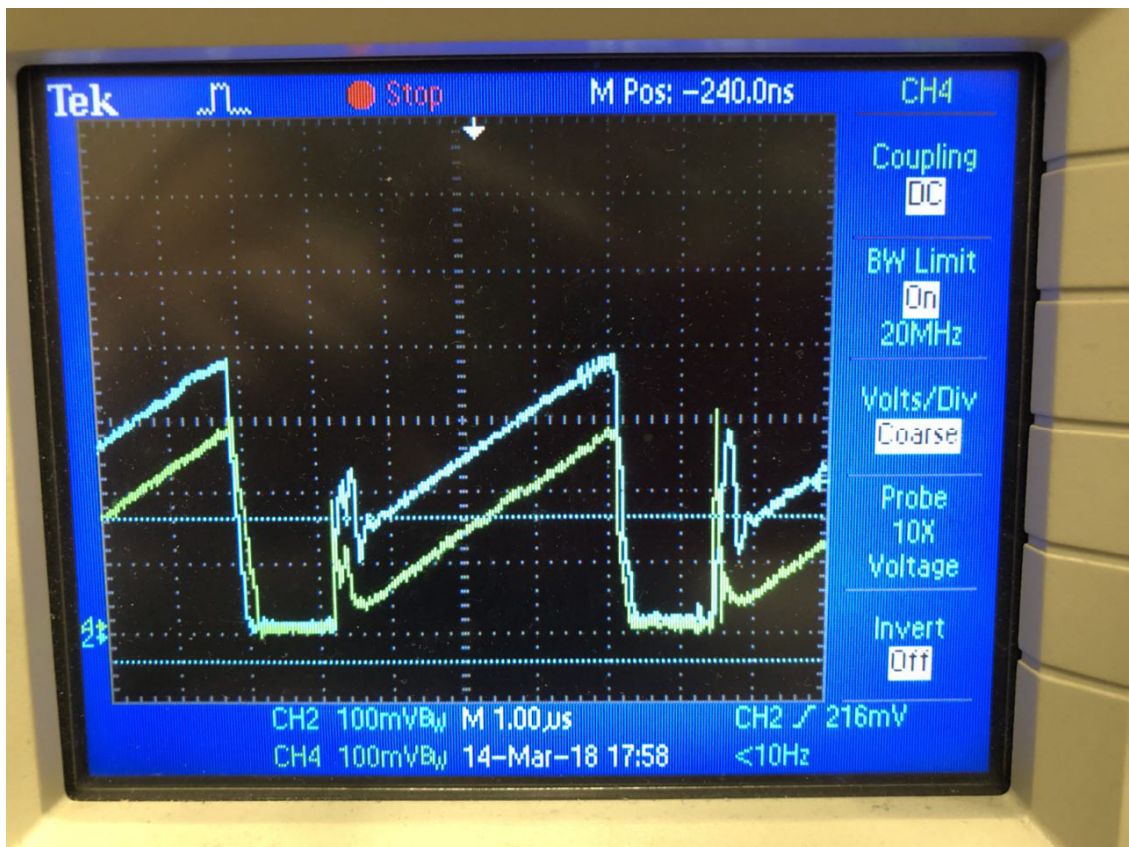
Figure 2 – CS signals, total output current is 70 A
