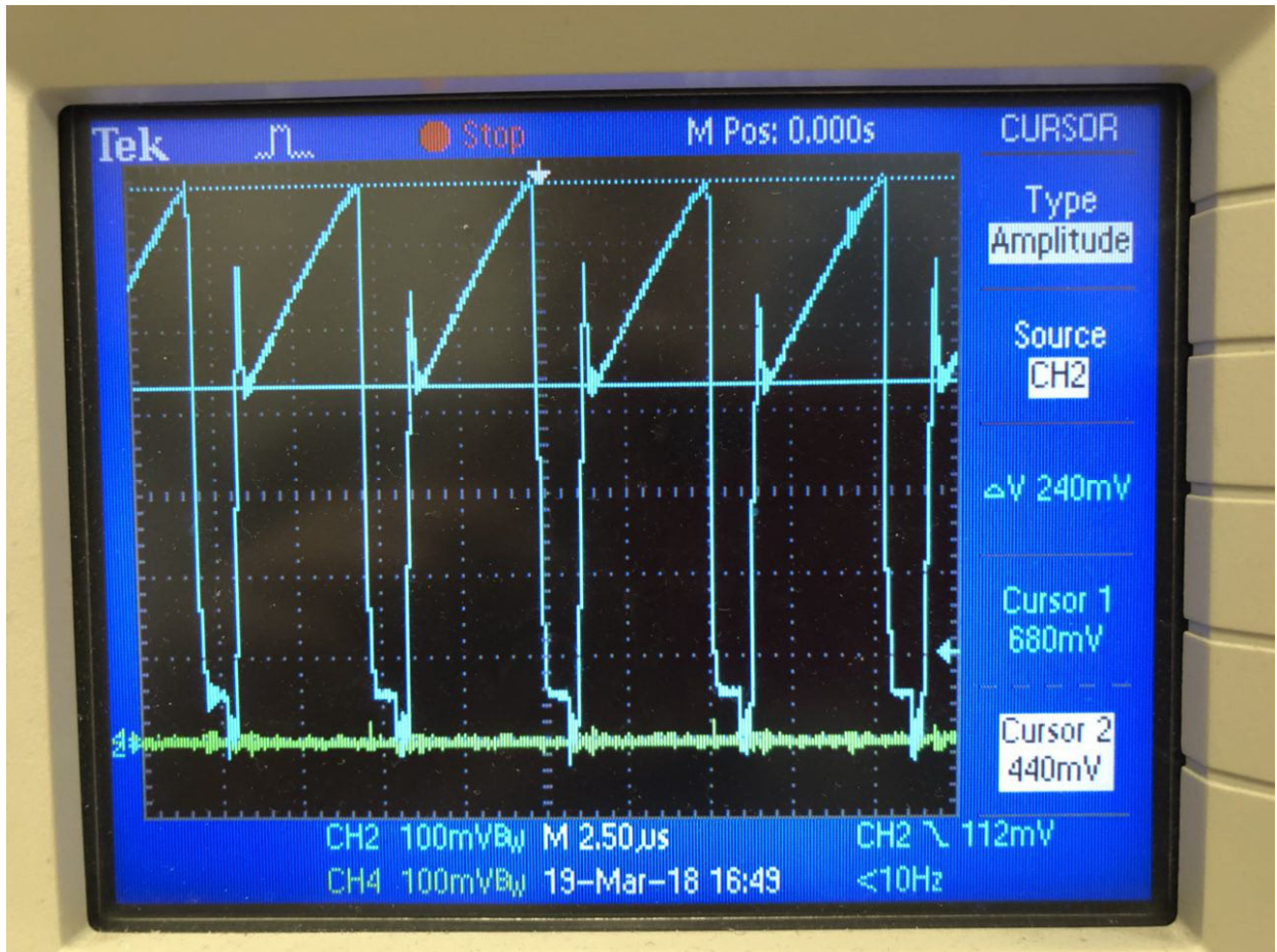
Figure 5 – CS signal of master converter when it works alone on 81 A load
