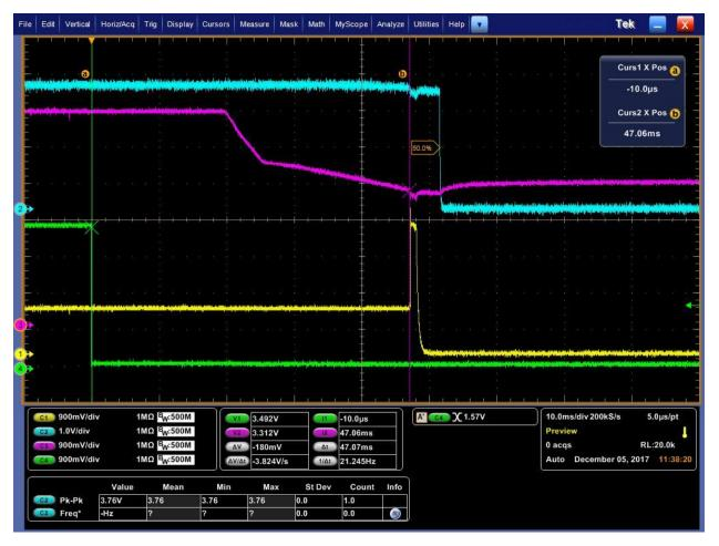
Power Off faulty sequence. The +1.1V (core rail) can be seen shutting up to 3.5V for about 840uS !!!!!!. This happens most likely due to wrong internal PMIC design or badly PMIC misbehaving for Vpmic (VINDCDCx...) at or approaching UVLO (3.3V). Clearly seen above.....
