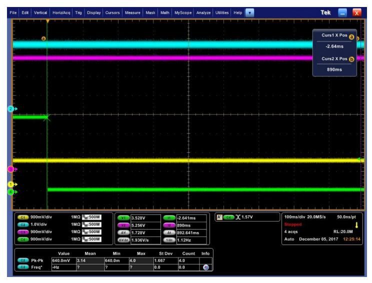
Power OFF sequence WAS initiated after 900mS after PWR\_EN = LOW; Please notice the Vin PMIC (VINDCDCx) is kept at 5.2V. Also, at this time the scope was set with 100ms/div and unfortunately the rails going down was not captured but I can tell for sure they eventually went down...!!!!!
