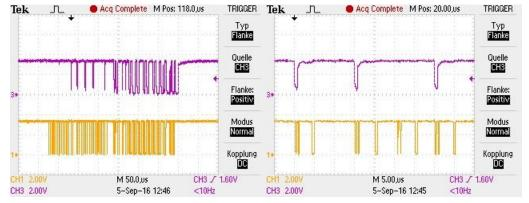
The cells are also connected like in the datasheet and when I push S1 I can measure that the TIDA-Board enters from ship mode to the normal mode. There are signals on the I2C Interface.
