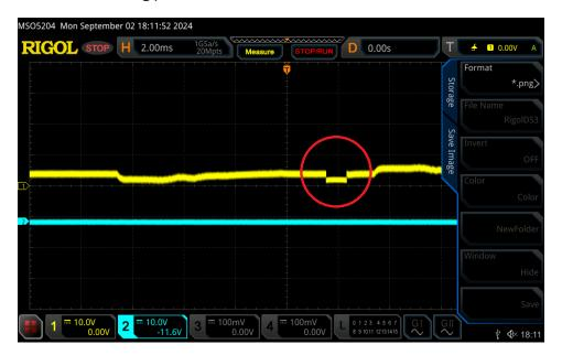
Meanwhile at Vcc = 27.85V, much shorter pulses are observed:
