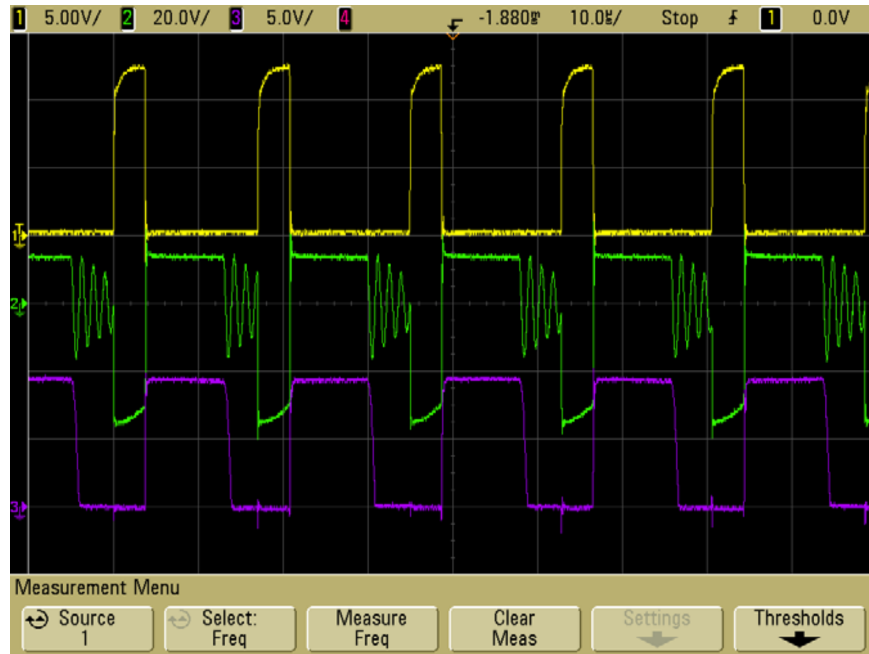
Ch1: Primary-Side FET Gate Drive, Ch2: Transformer Auxiliary Winding, Ch3: Flip-Flop based T_{off} Detector
