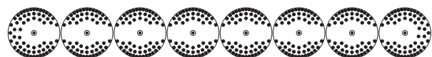
Figure 12. AC current distribution due to proximity effect for a single-layer winding, with all currents flowing in the same direction.
