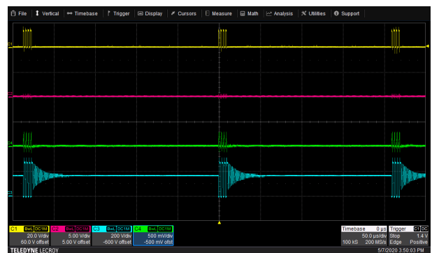
Figure 8-14. Typical Waveform in SBP2 Operation Yellow = PWML, Red = PWMH, Green = Transformer Primary Winding Current (0.2 V/A), Blue = Switch Node Voltage
