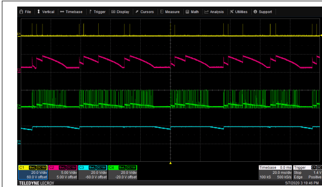
Figure 8-29. Boost Operation at 5 V OUT and No Load (Yellow = PWML, Red = BIN, Green = BSW, Blue = VDD)
