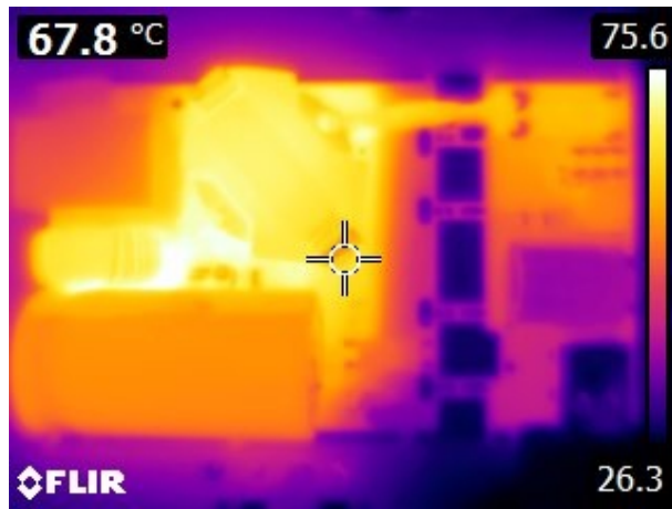
Figure 8-46. V_{IN} = 90 V_{AC} , Top Side (Transformer: 75.6 °C)
