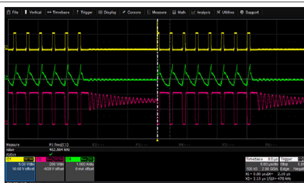
Figure 8-8. Maximum switching frequency about 240 kHz (Yellow = PWML, Green = Transformer Primary Winding Current, Red = Switch Node Voltage)
