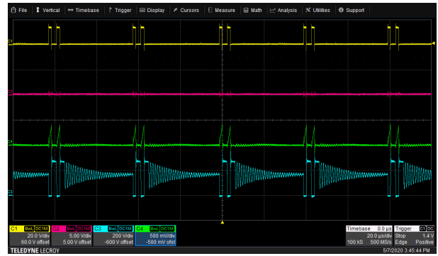
Figure 8-12. Typical Waveform in LPM Operation Yellow = PWML, Red = PWMH, Green = Transformer Primary Winding Current (0.2 V/A), Blue = Switch Node Voltage
