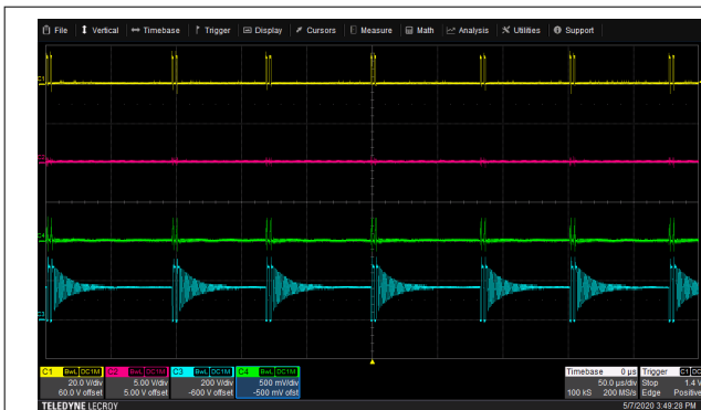
Figure 8-13. Typical Waveform in SBP1 Operation Yellow = PWML, Red = PWMH, Green = Transformer Primary Winding Current (0.2 V/A), Blue = Switch Node Voltage
