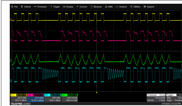
Figure 8-11. Typical Waveform in ABM Operation Yellow = PWML, Red = Vgs of SR MOSFET, Green = Transformer Primary Winding Current (0.2 V/A), Blue = Switch Node Voltage
