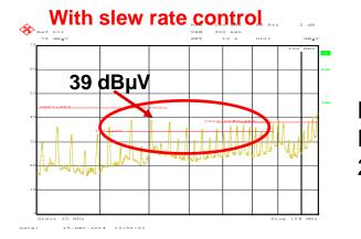
Measured on LM5140 standard EVM: 2.2 MHz, 3.3 V/5.0 Vout
