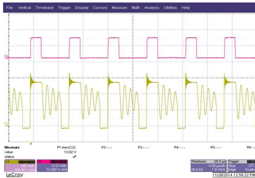
Figure 13. C1 = V_{SW} , C2 = V_{DRV} 115 V, 15 W
