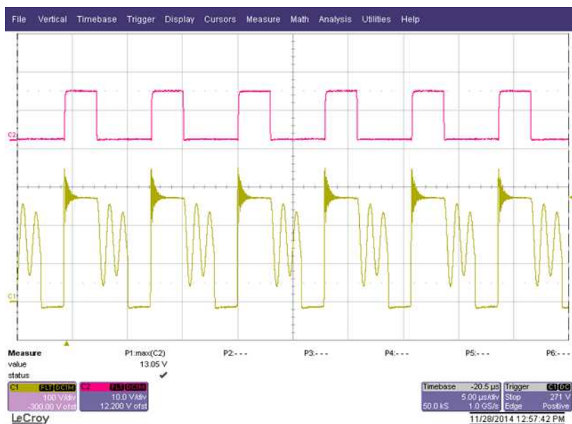
Figure 12. C1 = V_{SW} , C2 = V_{DRV} 230 V, 30 W
