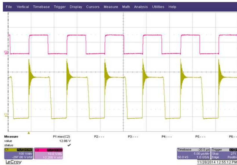
Figure 9. C1 = V_{SW} , C2 = V_{DRV} 115 V 65 W
