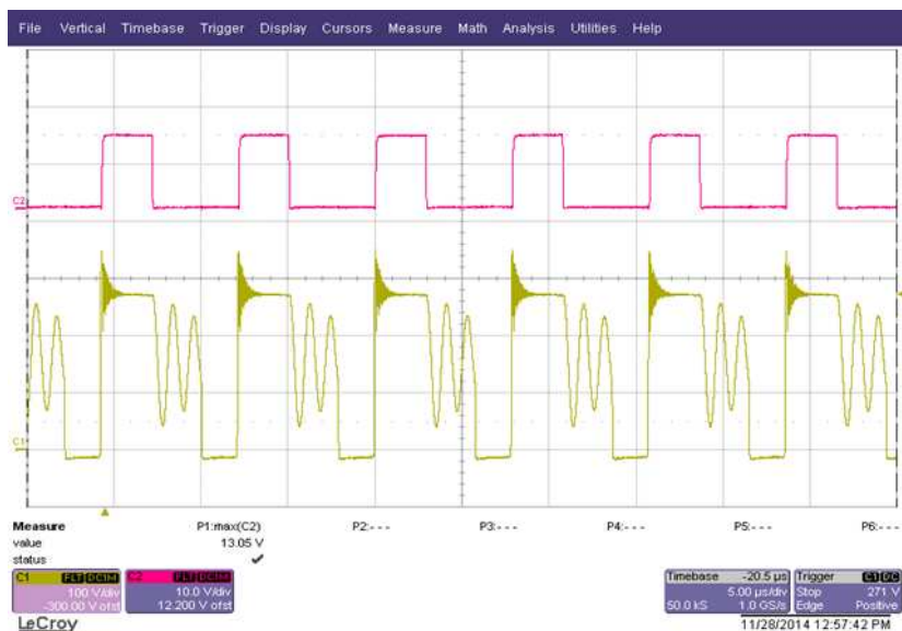
Figure 11. C1 = V_{SW} , C2 = V_{DRV} 115 V, 30 W
