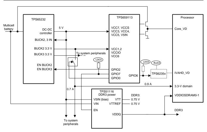
Figure 2. Example Power Solution With TPS659113
