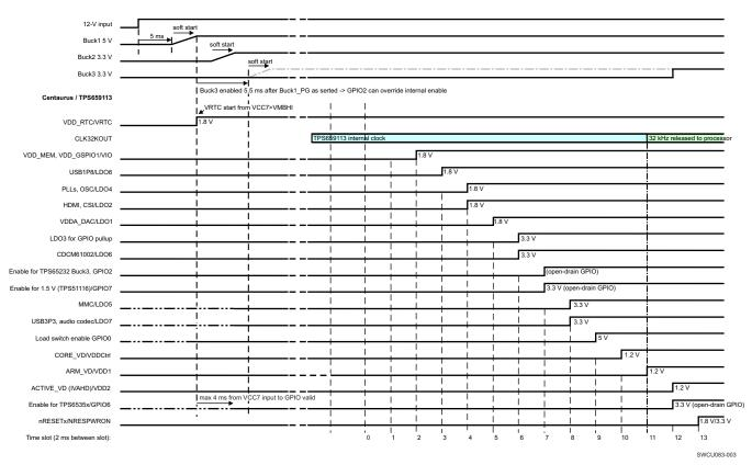
Figure 3. Power-Up Sequence Timing Diagram
