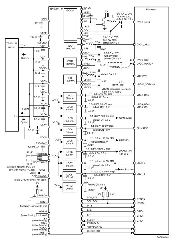
Figure 1. Processor Connection With TPS6591133
