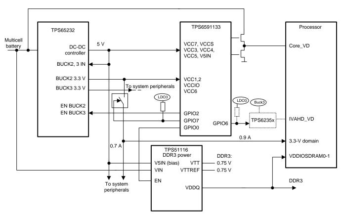
Figure 2. Example Power Solution With TPS6591133
