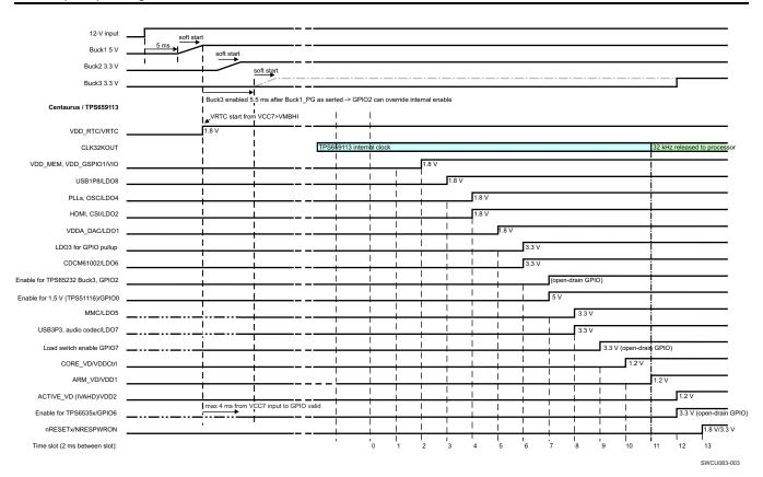
Figure 3. Power-Up Sequence Timing Diagram
