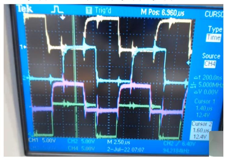
Vgs-Q2 (QA) and Vgs-Q3 (QD) are phase shifted more for smaller load currents compared to larger load currents. So, after Q2 turns OFF, for smaller load currents Q3 will turn off after a longer interval while for larger load currents Q3 will turn off after a shorter time interval, as seen for Iload = 25A below. Hence, tAFSET will be load dependent even with a fixed delay approach.
