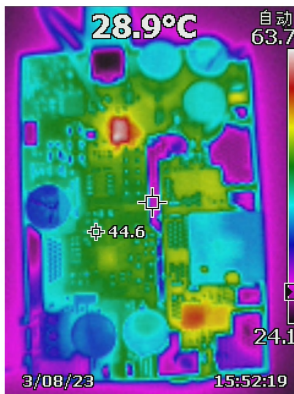
Figure 2-4. Charge Mode Thermal 20 Vsys to 7S Vbat
