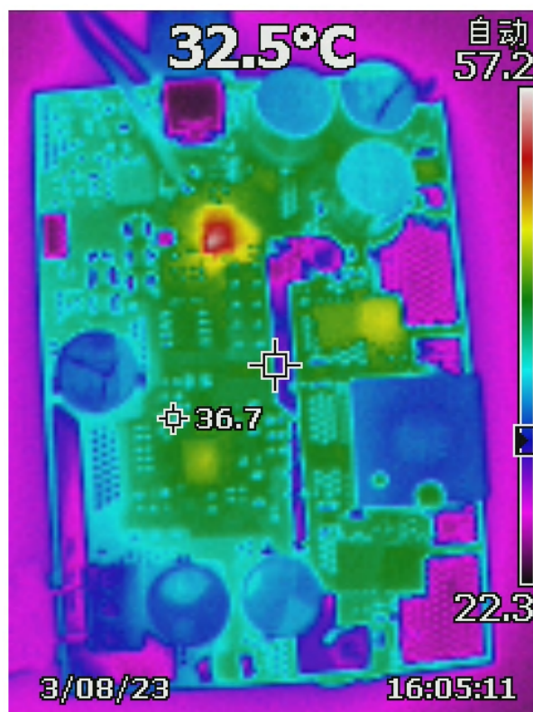
Figure 2-5. Charge Mode Thermal 20 Vsys to 4S Vbat
