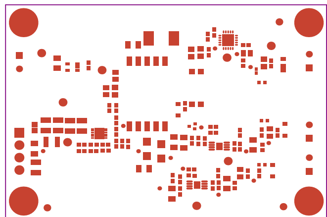
Figure 22. Top Solder Mask
