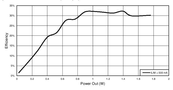
Figure 6 TIDA-00329 Efficiency with bq51003
