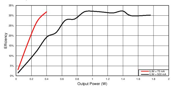
Firure 7 TIDA-00329 Efficiency versus Current Limit Setting (ILIM)
