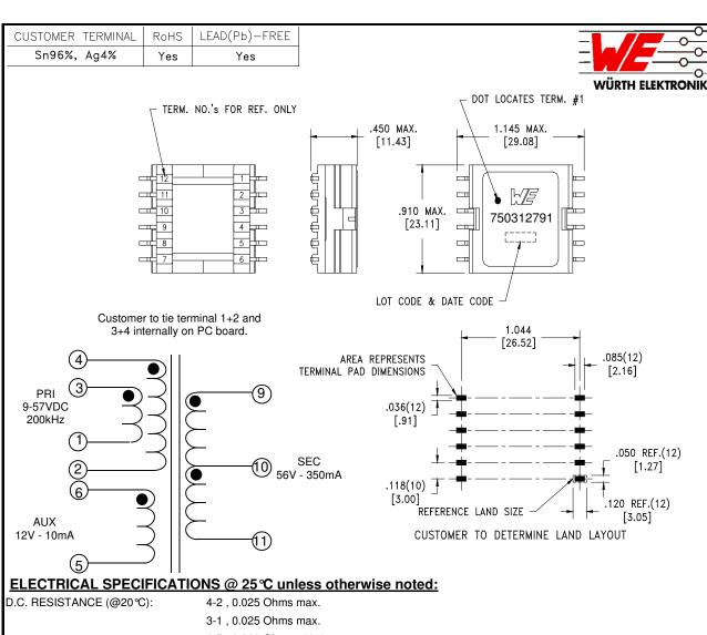
3-1 , 0.025 Ohms max. 6-5 , 0.260 Ohms ±10%. 9-11 , 0.250 Ohms ±10%.
