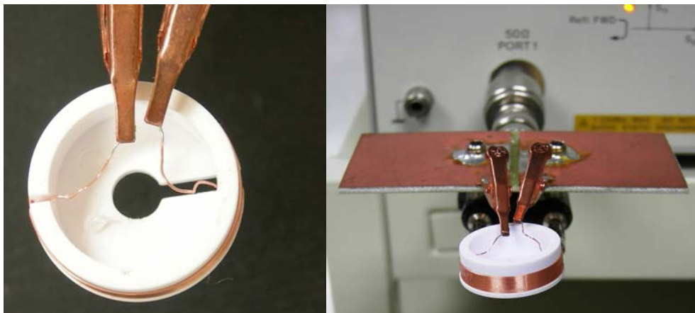
Figure 5. Measuring the Inductor with the Fixture
