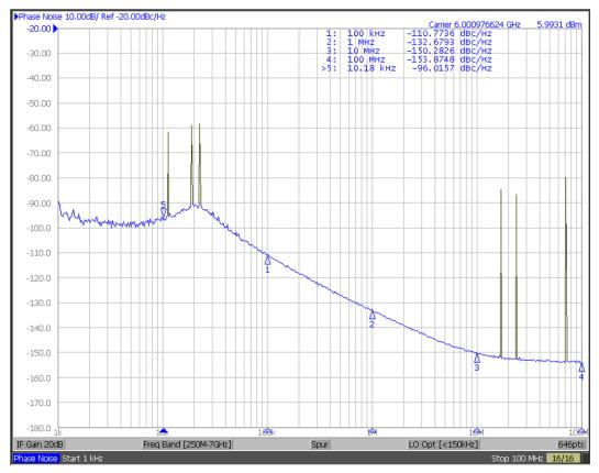
Figure 16. Spur Reduction by Setting the Reference Frequency to 102 MHz (No Spur at 1-MHz Offset)
