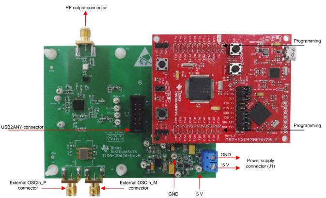
Figure 4. TIDA-00626 PCB Connectors
