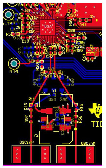
Figure 17. Layout Example for Input Reference and LMX2592
