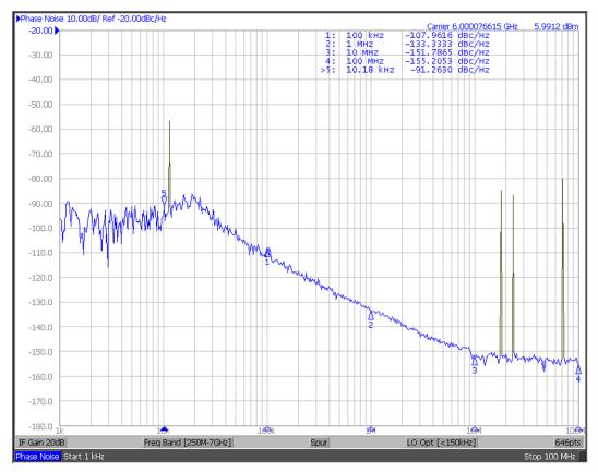
Figure 14. Spur Reduction by Setting the Reference Frequency to 102 MHz (No Spur at 100-kHz Offset)
