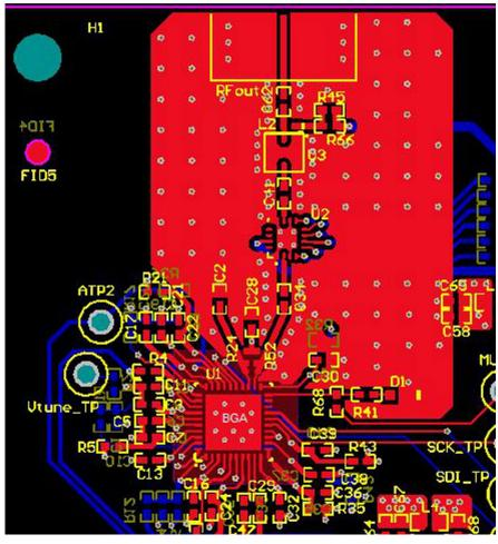
Figure 18. Layout Example for Output Section
