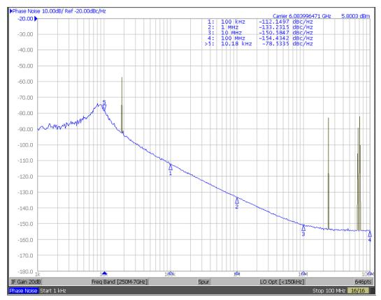
Figure 12. Spur Reduction by Setting the Reference Frequency to 102 MHz (No Spur at 10-kHz Offset)
