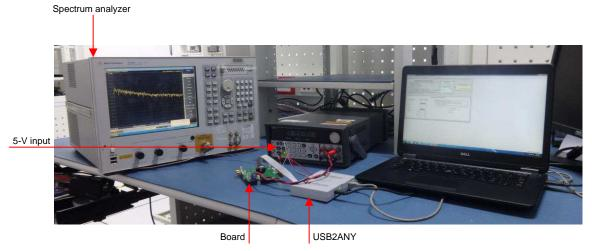
Figure 8. TIDA-00626 Test Setup
