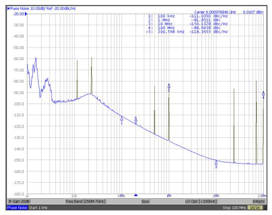
Figure 15. Spur at 1-MHz Offset From 6001-MHz Carrier due to VCO OSCin Coupling
