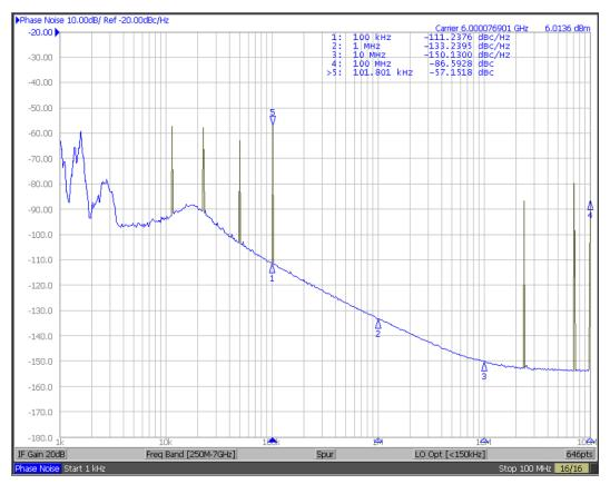
Figure 13. Spur at 100-kHz Offset From 6000.1-MHz Carrier due to VCO OSCin Coupling
