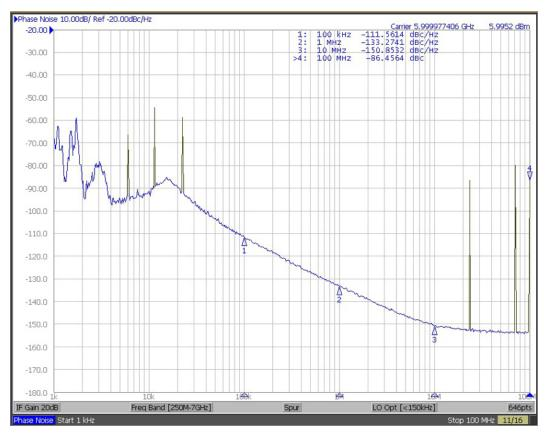
Figure 10. 6-GHz Output—Closed-Loop Phase Noise
