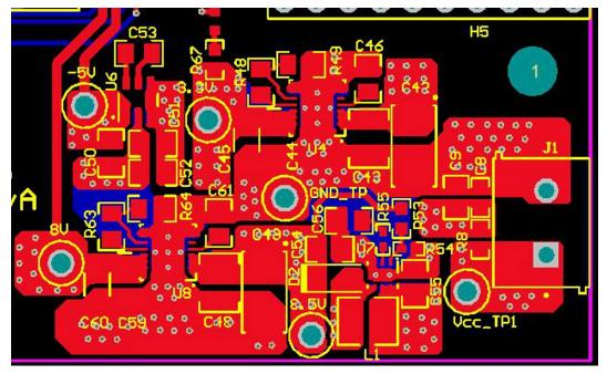
Figure 19. Layout Example for Power Supplies
