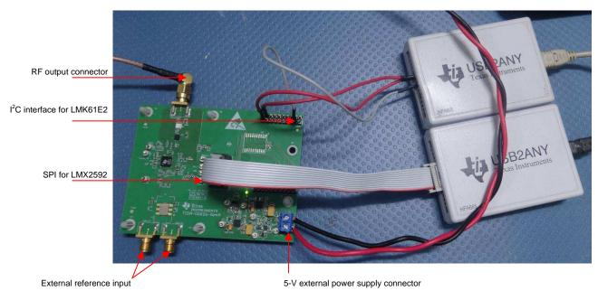
Figure 9. LMX2592 and LMK61E2 Programming Using TICS PRO GUI and CodeLoader 4 Using USB2ANY
