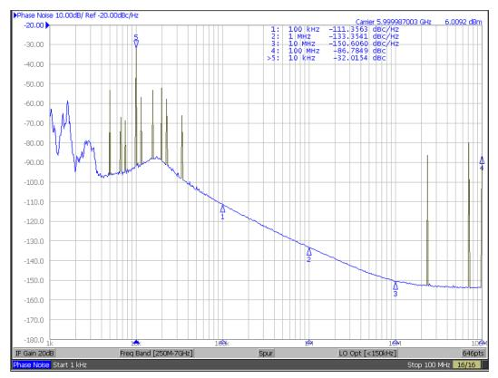
Figure 11. Spur at 10-kHz Offset From 6000.01-MHz Carrier due to VCO OSCin Coupling
