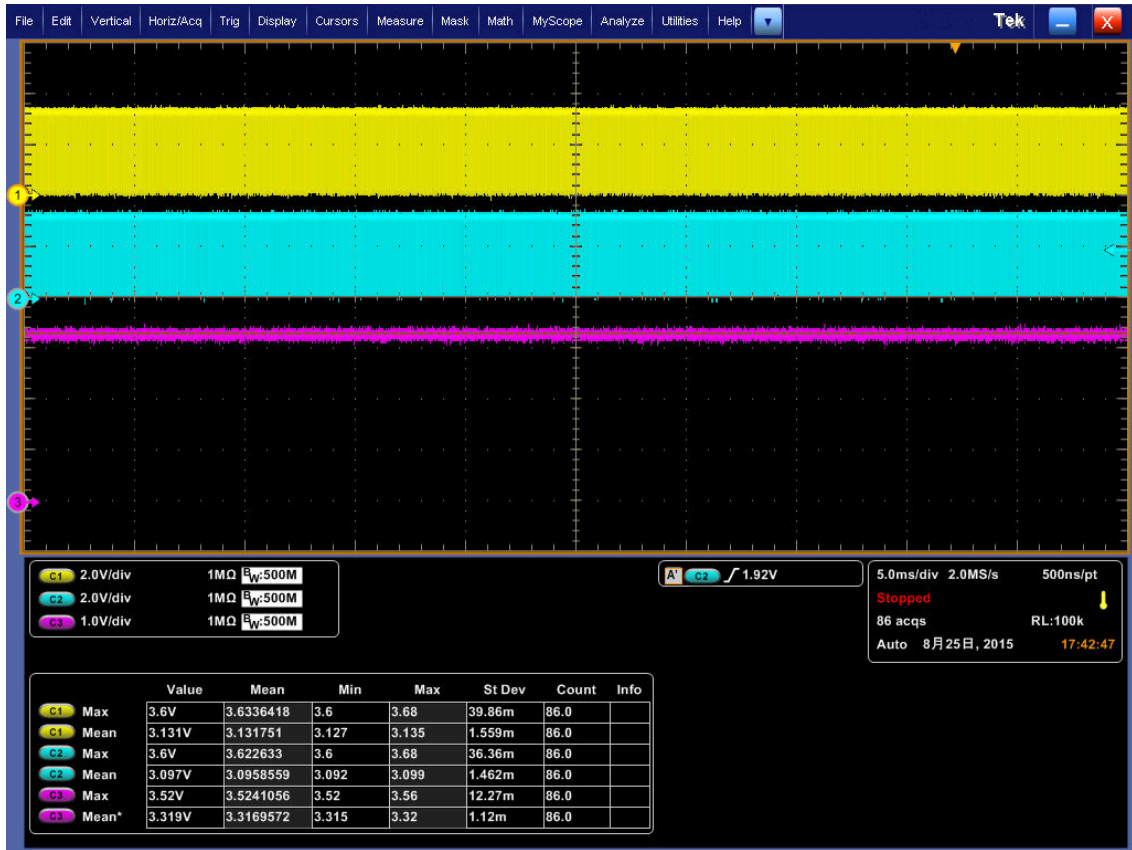
Fig. 8. OUT1 (CH1) , OUT2 (CH2) , REF 端子 (CH3) 電圧波形 (横軸 5msec./div.)
