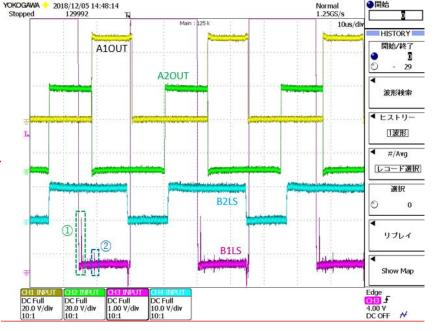
1.5V: After B1LS turns off(Cause unknown(noise))20.3V: It occurs synchronized with Aout1, Aout2 falling.
