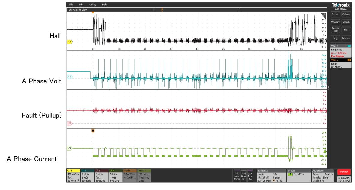
Retry is repeated even if Align Target Position is reached. Fault does not occur, A\_Align current is set value (10A), abnormal excess current cannot be observed.
