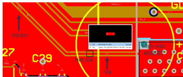
Figure 45. Net Tie High-Side MOSFET Drain
