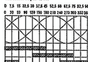
线反电势与霍尔相位关系图 (顺时针) Relation between phase EMFs and hall sensor outputs at CW
