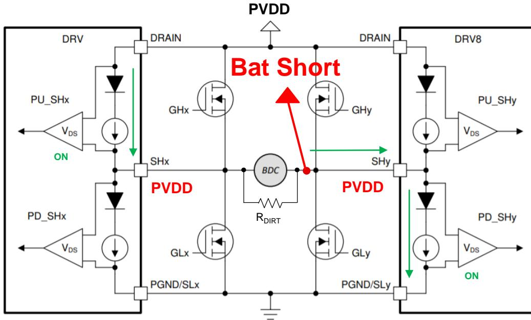
Battery Short Circuit Fault Detected:
