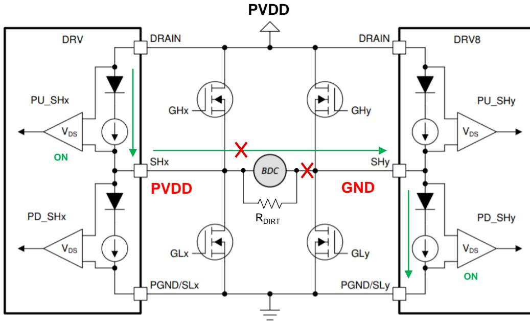
Open Load Fault Detected:
