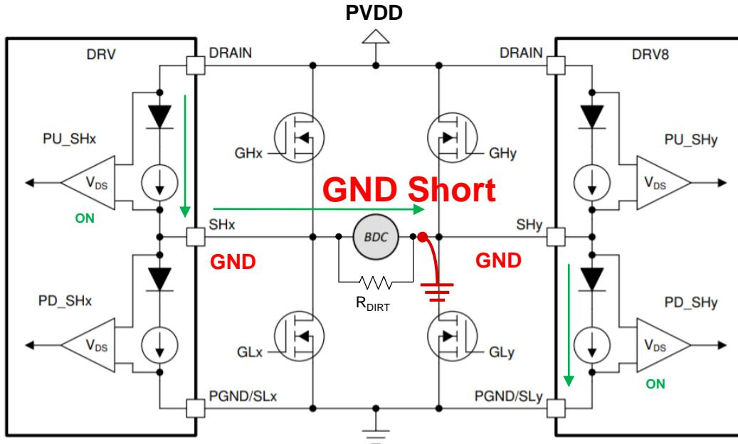
GND Short Circuit Fault Detected:
