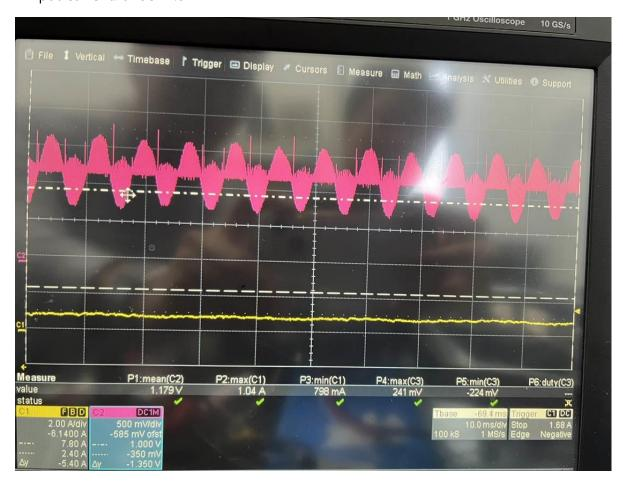
(CH1: Input current of DRV8316, CH2: SOA, A: U phase, B: V phase, C: W phase)
