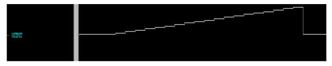
Notice in the waveform above, there are 20 step sizes ramping the waveform from 0x00 to 0x3F
