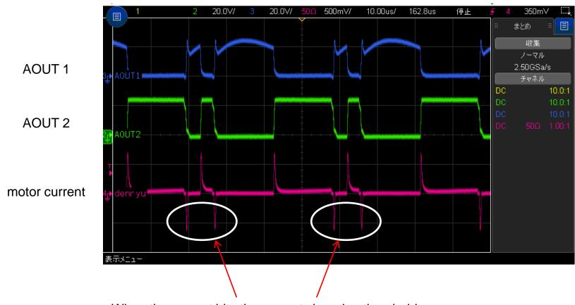
When the current hits the current chopping threshold, the current flow reverse in a moment.
