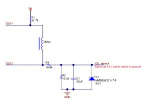
Open Load detection circuit
