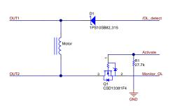
Open Load detection circuit
