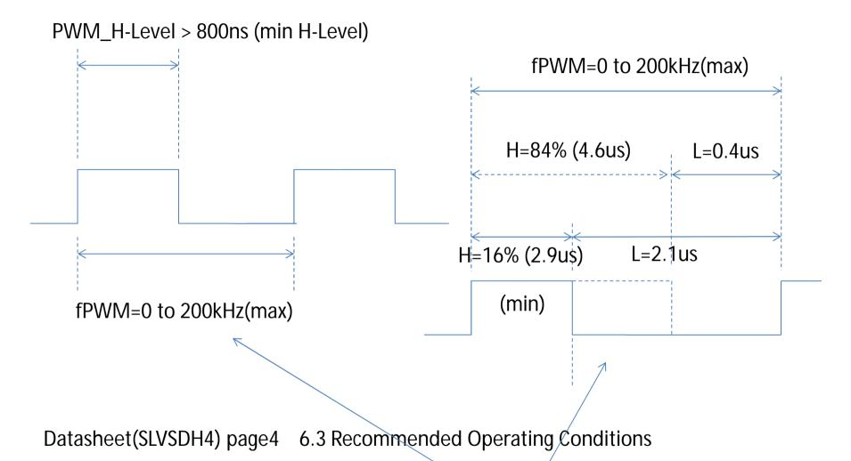
(1) The voltages applied to the inputs should have at least 800 ns of pulse width to ensure detection. Typical devices require at least 400ns.
