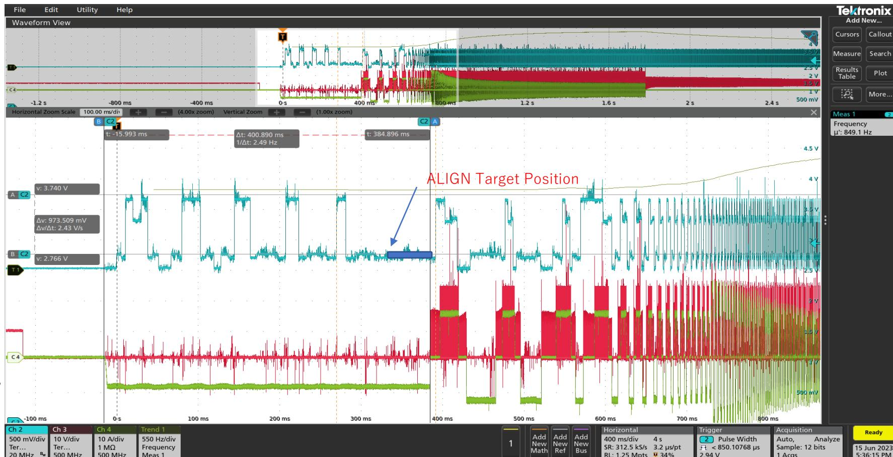
AlignMode causes the motor shaft to move, but Retry does not occur.
