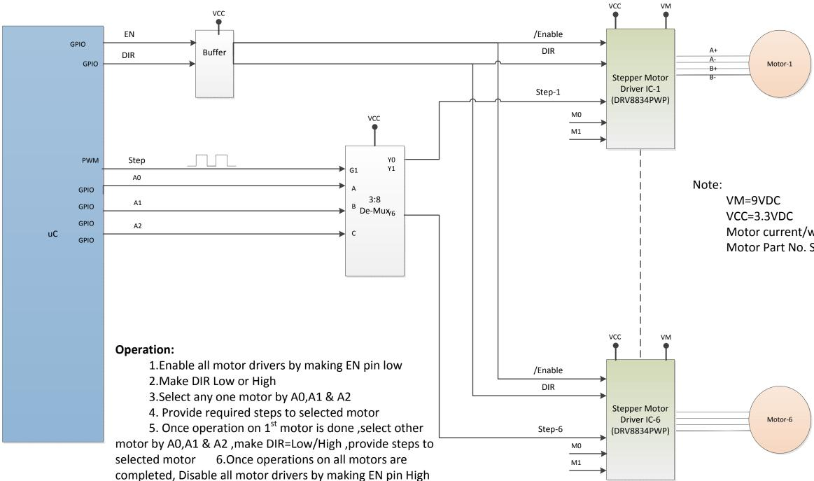
VM=9VDC VCC=3.3VDC Motor current/winding set to 180mA Motor Part No. SH2141-5541
