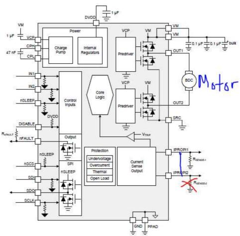
DRV8873 is just replace relays in our control box, which controll the Motor up and down.
