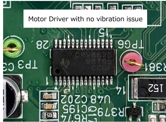
DRV8825 98TG5 CCGF is written on the surface of the package.
