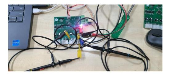
To validate the functionality of the DRV8231DSGR IC, the following oscilloscope test configuration was used:
