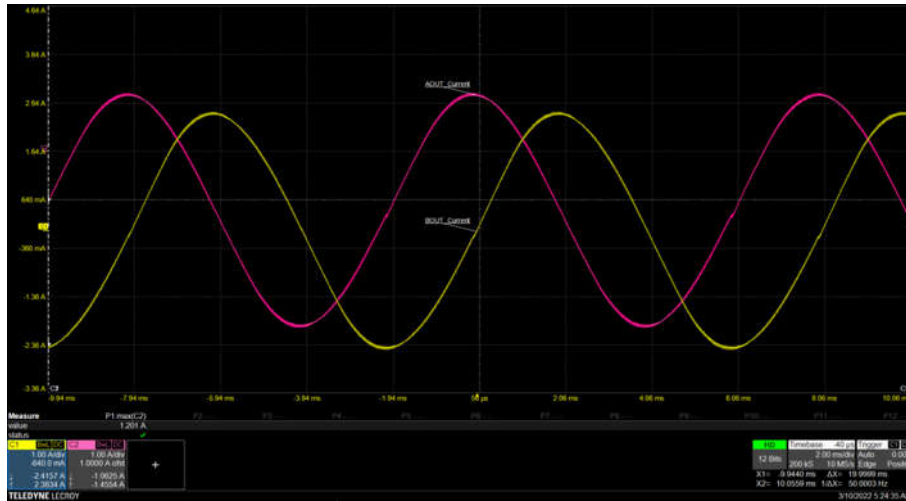
Figure 7-21. Coil Current Waveform with Silent Step Decay
