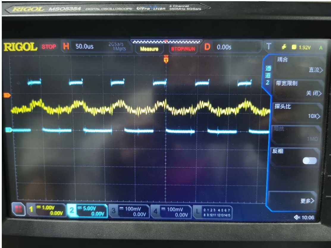
黄色-ISENA 蓝色-ISENB, 电流 420mA Yellow represents ISENA, blue represents ISENB, current 420mA
