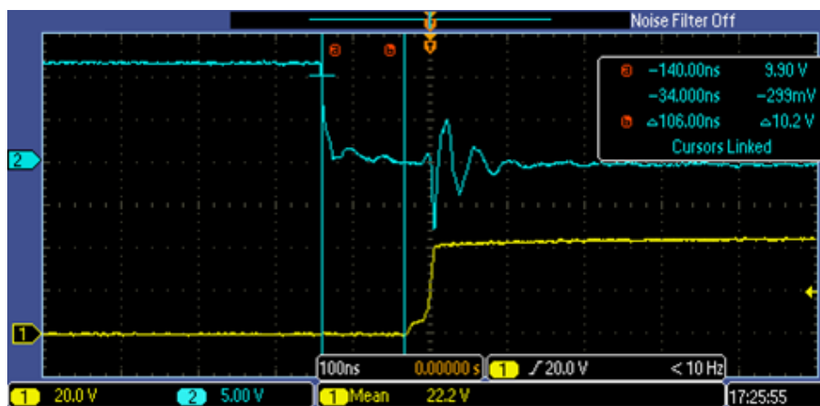
Figure 27. Dead Time Inserted by DRV8303 Measured at Falling Edge of Lower FET PWM
